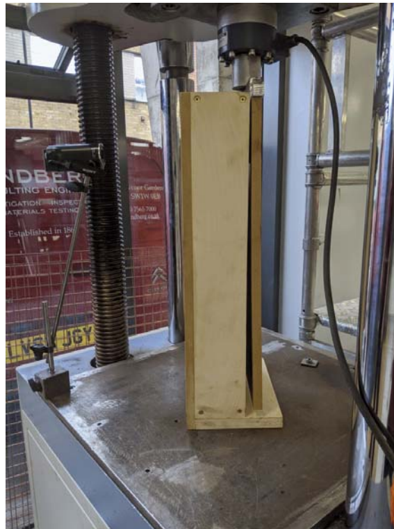
Photograph 1 A view showing the general test setup for shear testing of four type 2 Button-fix fixings.
