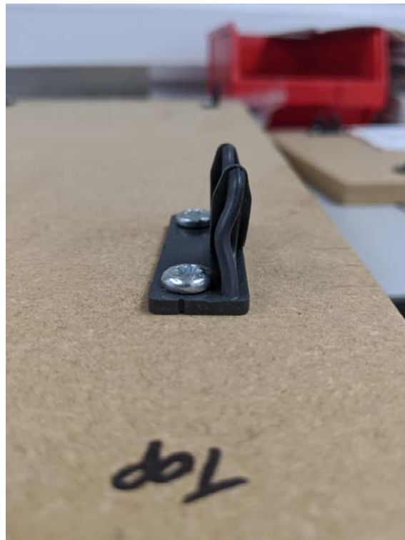
Photograph 2 A view showing the general condition of the fixing after a shear test, with the top jaw of the fixing deformed.
